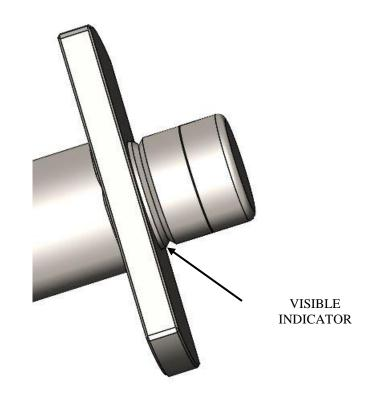
2. Insert laterally the tooling on the connector
