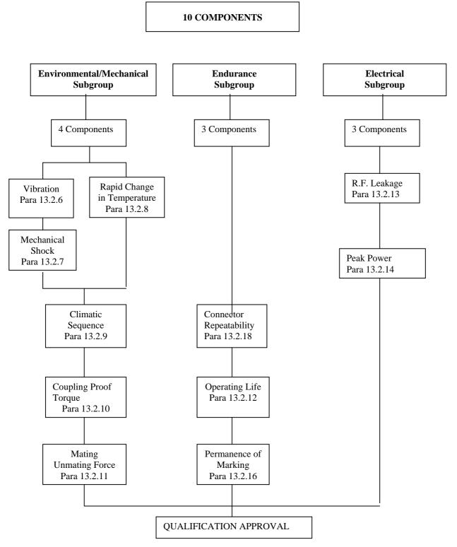
The number of failures allowed is 1 per subgroup but the cumulative number of failures for qualification for all three subgroups is also 1
