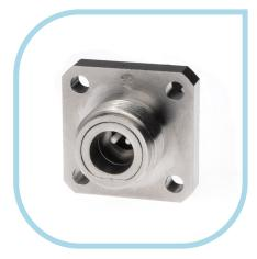
Dedicated to outdoor optical connections for FTTA (Fiber to the Antenna), RXF connectors feature a Type N mechanical interface with IP68 sealing and low insertion loss. RXF connectors are available in 2 or 4 channels, in MultiMode or SingleMode UPC versions.
