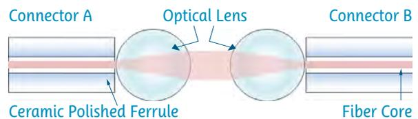
EB technology offers a contactless connection which increases the number of mating cycles compared to connectors based on Physical Contact technology. Due to the signal being expanded, the connection is also less sensitive to particular contamination and supports an easier cleaning process. This makes it the ideal choice for demanding applications requiring ease of maintenance in highly contaminated environments.
