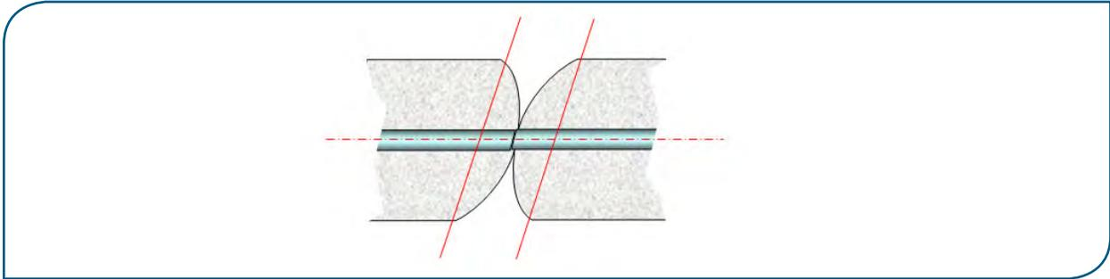
This type of technology achieves excellent Return Losses (>65 dB), useful to protect sensitive light sources like laser diode from optical feedback.
