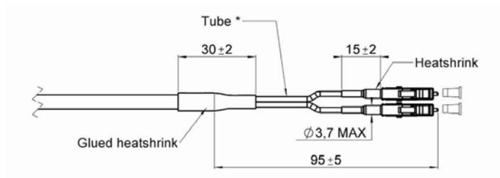
\*Tube must be flexible enough to guarantee the bending radius of the fiber.
