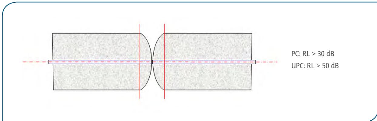
The UPC (Ultra Physical Contact) polishing may be required for SingleMode fibers: the geometry is the same as PC and leads to the same level of insertion losses but the quality of polishing is higher and provides Return Losses of 50 dB (compared to 30 dB in PC).
