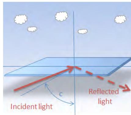
Light is totally reflected because its angle of incidence is superior to the critical angle.
