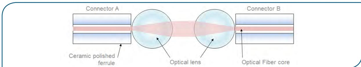
Most of the time, no adaptor is required for that type of assembly: the plugs are able to connect to each other.
