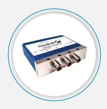
To meet market demands for V band equipment, Radiall has extended the 67 GHz offer with the development of DP3T & SPDT Terminated Coaxial Switches that operate up to 67 GHz. Fitted with 1.85 mm connectors, these new switches are perfectly suited for 5G applications and other instrumentation applications.
