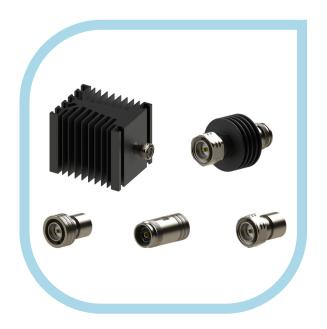
Following the commercialization of the 4.3-10 series of connectors, Radiall developed a global range of microwave components equipped with 4.3-10, including terminations up to 100W and attenuators up to 15W. These terminations are available from low power (2W) up to high power (100W) at 6 GHz maximum frequency and provide outstanding electrical performance.
