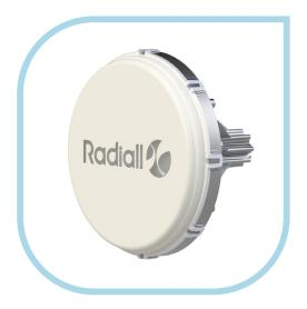
Radiall's V-Band mmWave antenna is perfectly suited for integration in new telecom systems, where small form factor and high gain are critical. This new solution provides 32 dBi bore sight gain from 57 to 66 GHz coinciding with the normal axis of the antenna. This feature helps to facilitate quick and easy alignment between radio units (optical technology or not), which is mandatory for applications such as small cells, backhaul/fronthaul links and WiGig.
