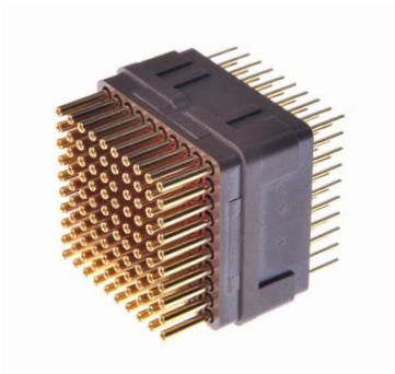
This solution offers a new monoblock insert available for size 22 PC tail contacts, in 100 and 150 points configurations. Molded in one piece and fitted with fixed contacts, it simplifies the manufacturing process to reduce cost and weight. The insert's unique design supports basic movement of the contacts inside the cavity to provide mechanical play offering a mating force similar to traditional Arinc 600 connectors.
