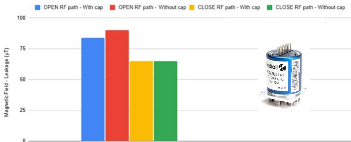
Figure 9 : Impact of cap on magnetic field leakage
