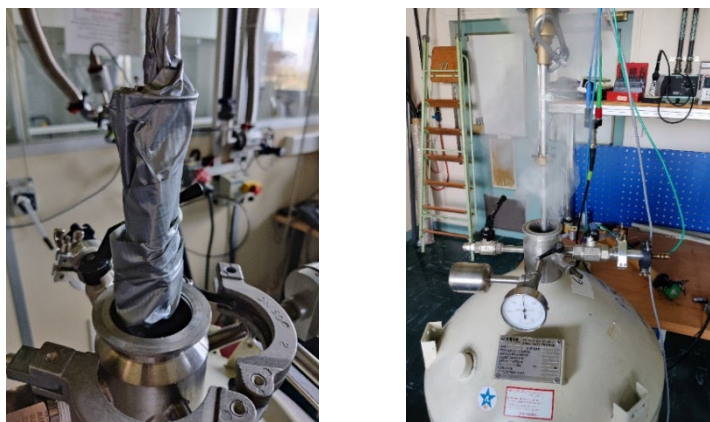
Figure 16 : Head protected with scotch tape plunged in a liquid Helium.
