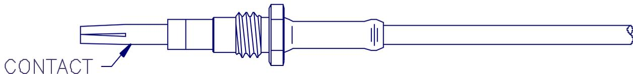
7. SOLDER CONTACT TO CENTER CONDUCTOR.
