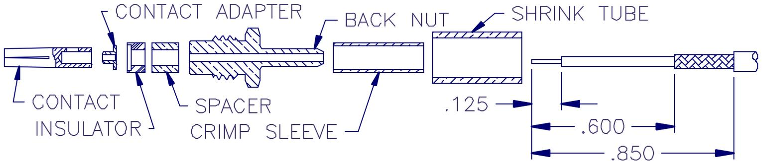
1. TRIM CABLE AS SHOWN. TIN END OF CENTER CONDUCTOR.
