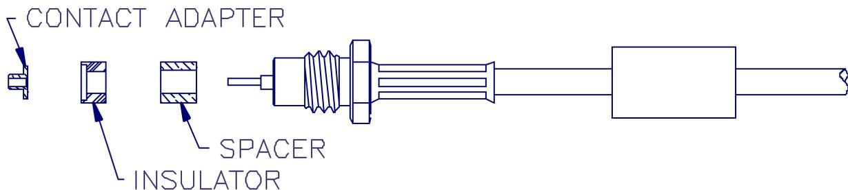
6. POSITION SPACER, INSULATOR THEN CONTACT ADAPTER OVER CABLE DIELECTRIC AND CENTER CONDUCTOR.
