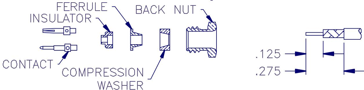
1. TRIM CABLE AS SHOWN. TIN END OF CENTER CONDUCTOR.
