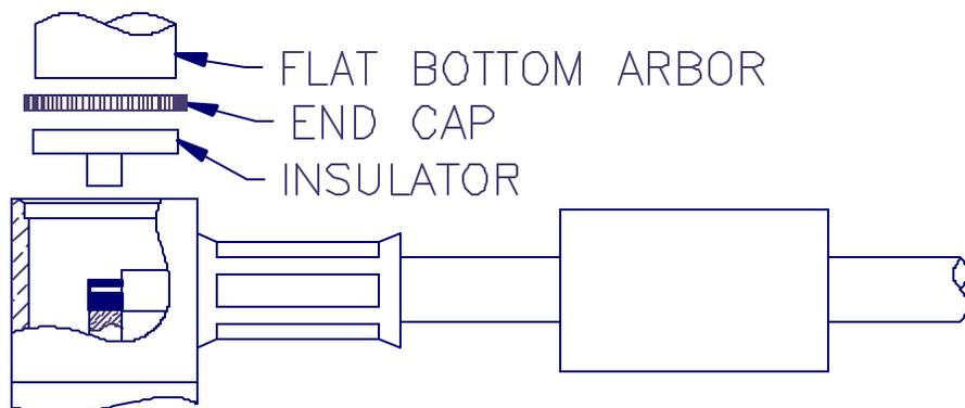
7. PLACE INSULATOR AND END CAP INTO CONNECTOR BODY AS SHOWN AND USE A .185" DIAMETER FLAT BOTTOM PUNCH TO PRESS CAP IN PLACE. CAP MUST BE BELOW SURFACE TO SEAT PROPERLY.
