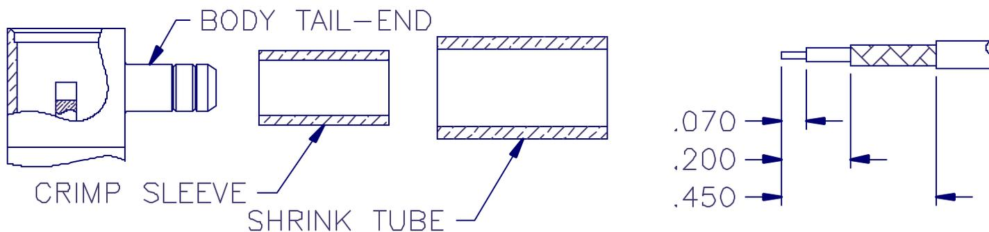
1. TRIM CABLE AS SHOWN. TIN END OF CENTER CONDUCTOR.
