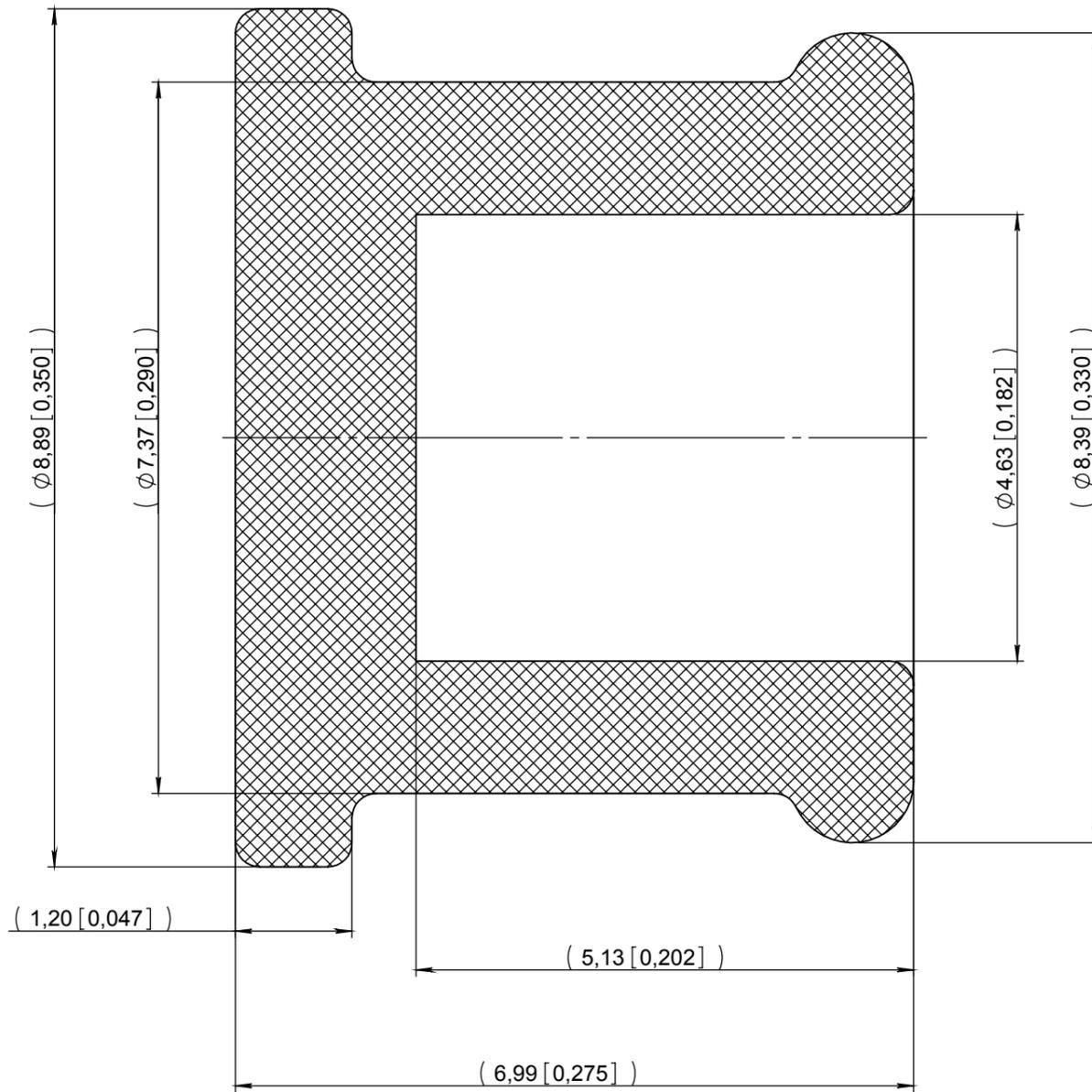
Material: Fluorosilicone elastomer
