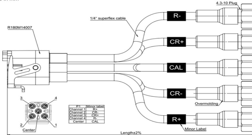
CONNECTORS DESIGNATION Connector 1: **MLOC5 PLUG** Connector 2: **4.3-10 PLUG**
