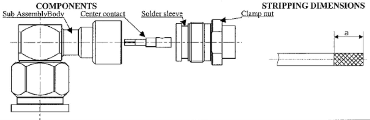
**1** Strip the cable. Slide the clamp nut onto the cable. Solder the ferrule onto the braid of the cable.
