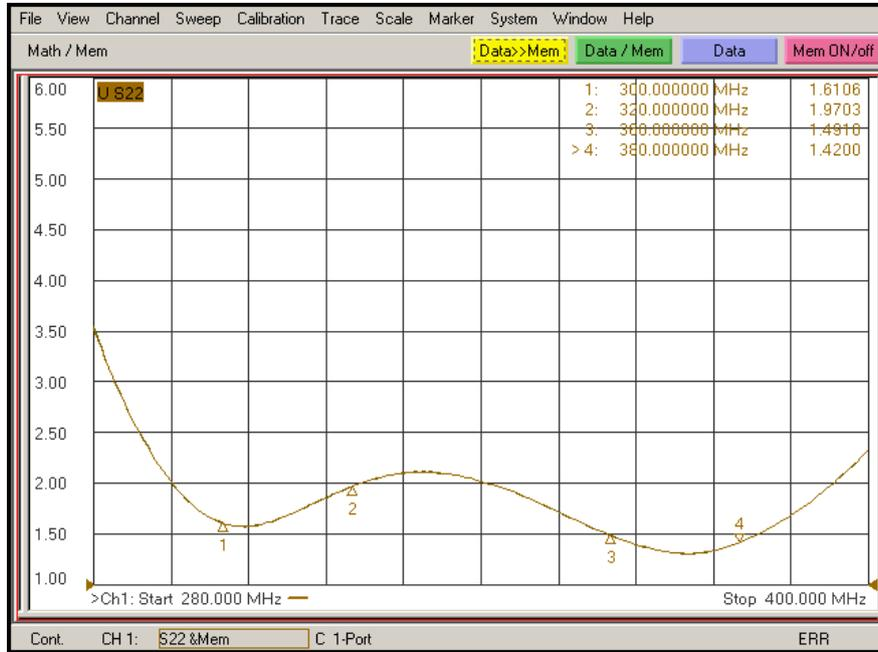
Figure 1: VSWR measured when mounted on man-pack chassis 1m above ground
