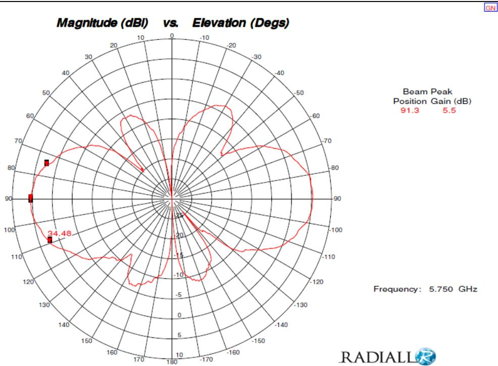
*Figure 6: Vertical Radiation Pattern @ 5750 MHz*
