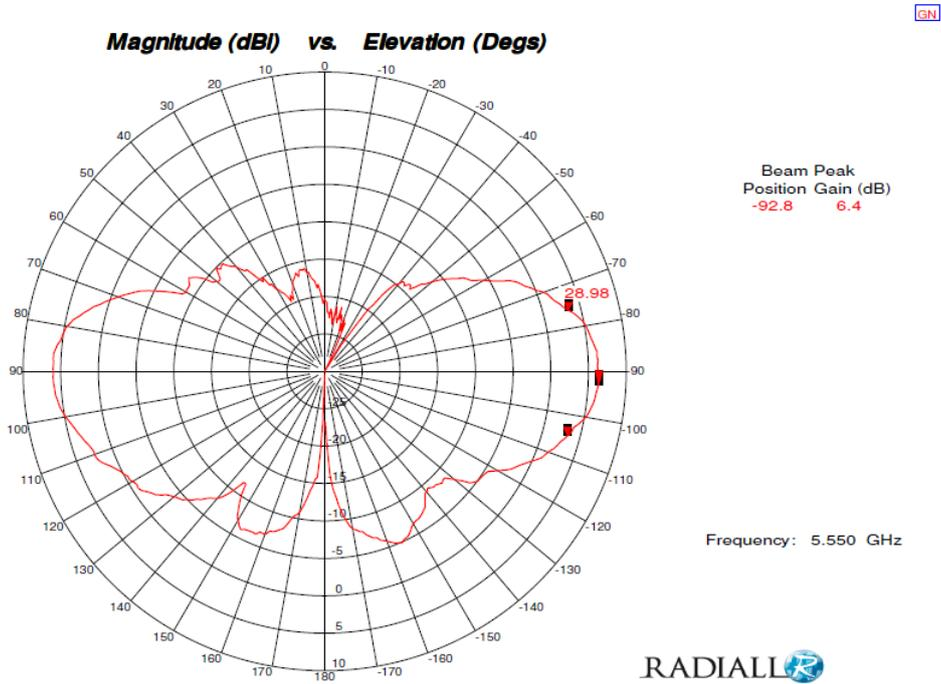
*Figure 5: Vertical Radiation Pattern @ 5550 MHz*
