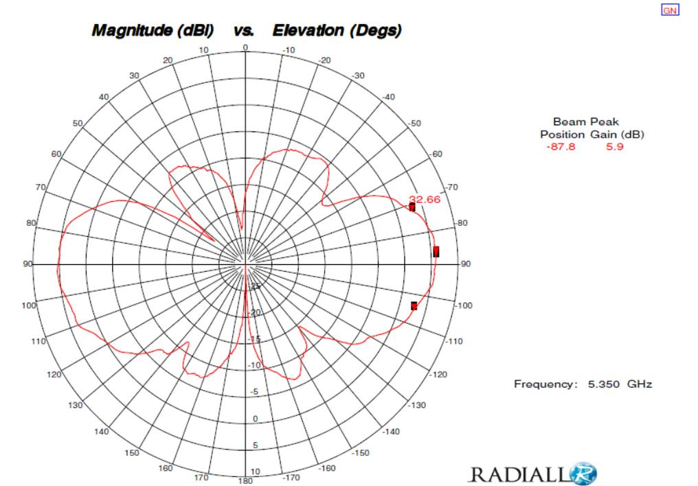
*Figure 4: Vertical Radiation Pattern @ 5350 MHz*
