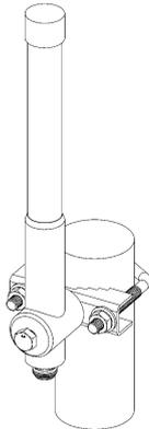
3. Wall mount antenna by placing antenna mount assembly against wall. **NOTE: Wall mount hardware (Not Included) must be adequate for the material it is going into. Do not use v-bolt for wall mount application.**
