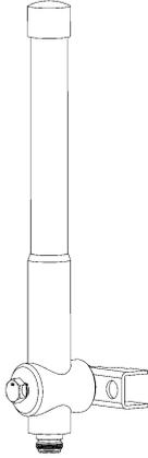
2. Position antenna mount assembly onto pole and install v-bolt. Install nuts and tighten using 13 mm wrench. Pole size .75 to 2 inch diameter.
