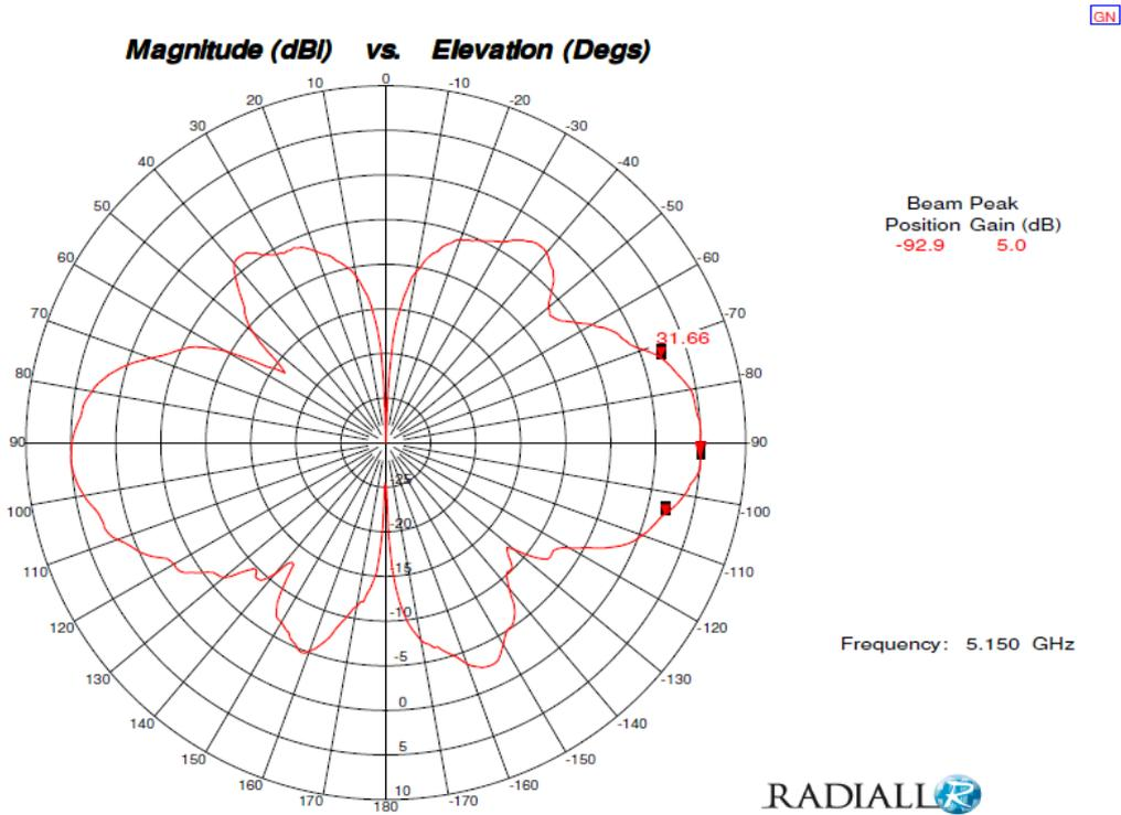
*Figure 3: Vertical Radiation Pattern @ 5150 MHz*
