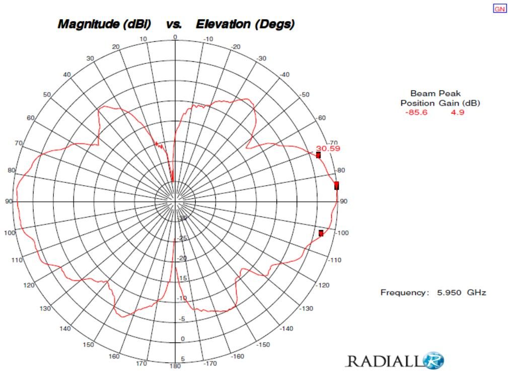
Figure 5: Vertical Radiation Pattern @ 5950 MHz
