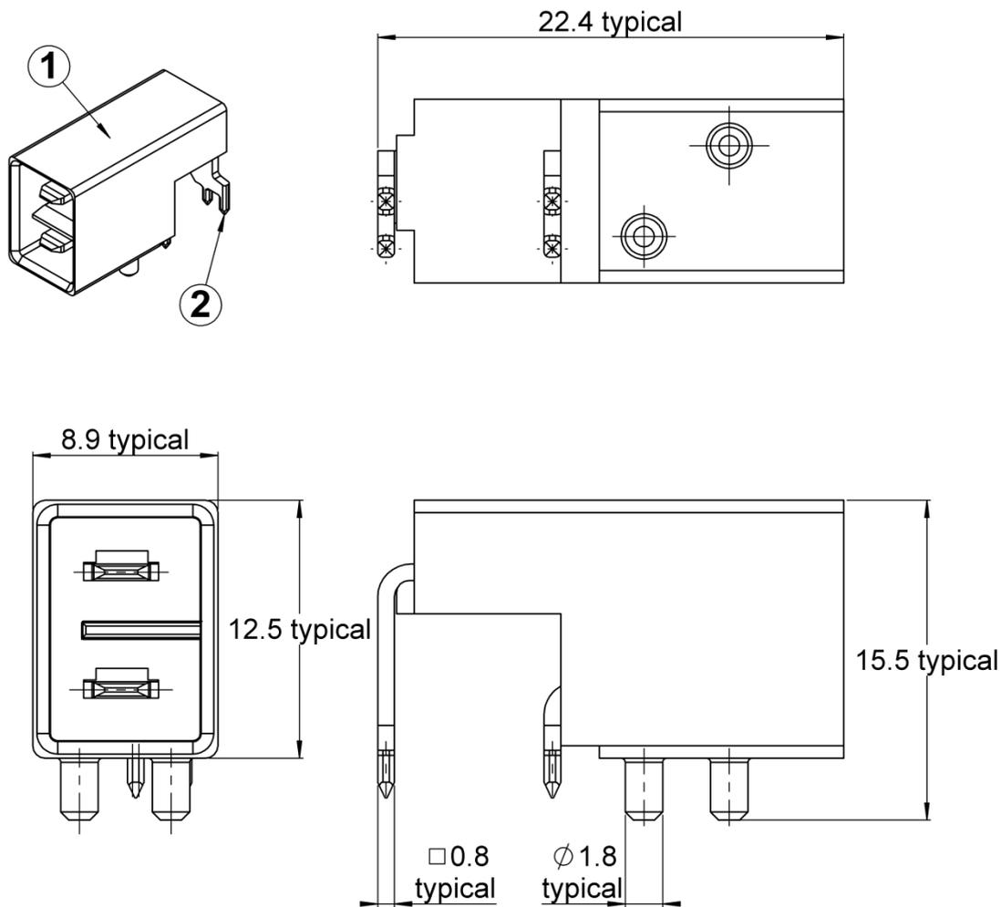
All dimensions are in mm. Unmarked tolerance is  $\pm 0.3$ mm
