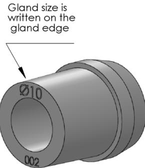
\*Cable diameter under the gland. If the cable has a sleeve, the diameter over the sleeve should be considered
