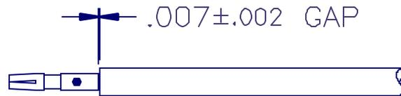
2. SOLDER CONTACT TO CENTER CONDUCTOR, LEAVING A GAP BETWEEN REAR OF CONTACT AND CABLE JACKET AS SHOWN.
