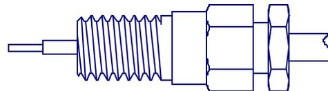
5. INSERT CABLE ASSEMBLY INTO BODY AND TIGHTEN NUT WITH A TORQUE OF 90-100 INCH OUNCES.
