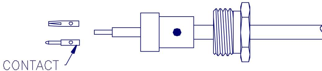
5. SOLDER CONTACT TO CENTER CONDUCTOR. CONTACT TO BE SEATED FLUSH AGAINST DIELECTRIC.
