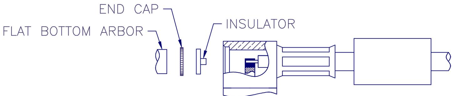
7. PLACE INSULATOR AND END CAP INTO CONNECTOR BODY AS SHOWN AND USE A .185" DIAMETER FLAT BOTTOM PUNCH TO PRESS CAP IN PLACE. CAP MUST BE BELOW SURFACE TO SEAT PROPERLY.
