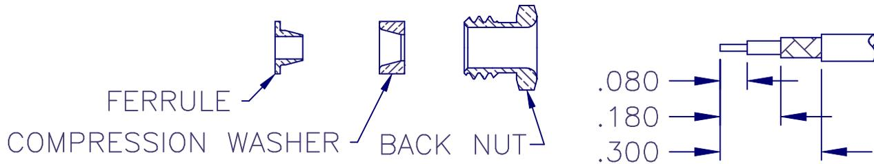
1. TRIM CABLE AS SHOWN. TIN END OF CENTER CONDUCTOR.
