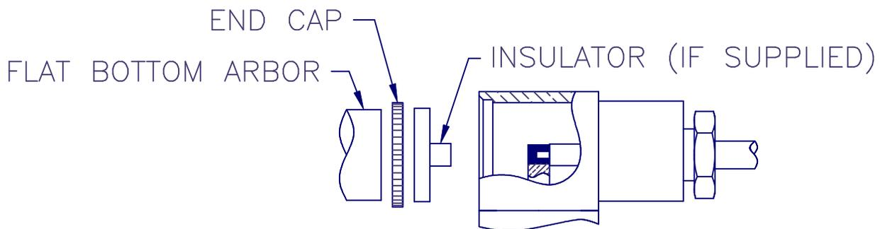
5. INSERT CABLE ASSEMBLY INTO BODY AND TIGHTEN NUT WITH A TORQUE OF 90-100 INCH OUNCES.
