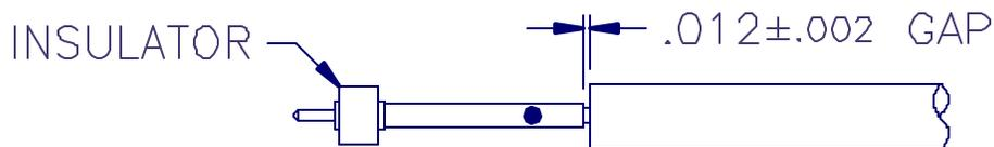
2. SOLDER CONTACT TO CENTER CONDUCTOR, LEAVING A GAP BETWEEN REAR OF CONTACT AND CABLE JACKET AS SHOWN.
