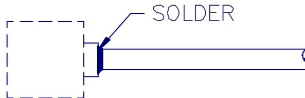
4. INSERT CABLE INTO BODY UNTIL IT BOTTOMS. CHECK THAT INSULATOR AND CONTACT MEET INTERFACE DIMENSIONS.
