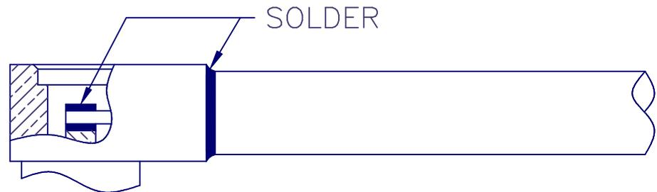
4. SOLDER CENTER CONDUCTOR TO CONTACT.
