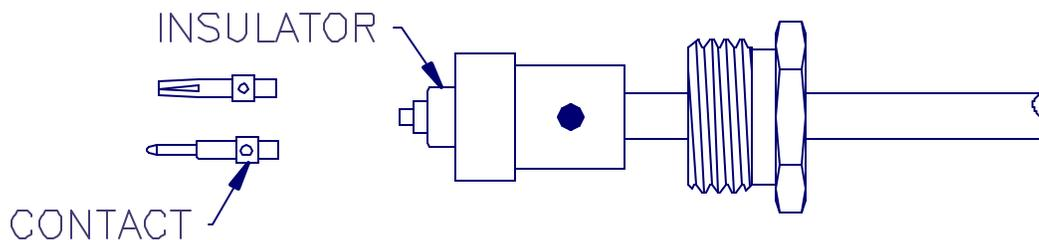
6. SOLDER CONTACT TO CENTER CONDUCTOR.
