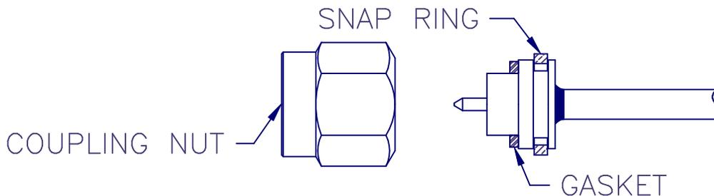
5. INSTALL SNAP RING AND GASKET ONTO CONNECTOR BODY.
