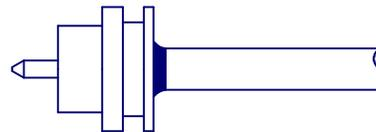
3. INSERT CABLE INTO BODY UNTIL IT BOTTOMS. CHECK THAT INSULATOR AND CONTACT MEET INTERFACE DIMENSIONS.
