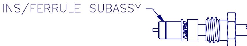
5. SLIDE INS/FERRULE SUBASSY ONTO CABLE, OVER DIELECTRIC AND UNDER BRAID. PUSH INTO WASHER UNTIL IT STOPS. IF NECESSARY TRIM EXCESS BRAID FLUSH WITH SURFACE OF COMPRESSION WASHER AND FLANGE OF FERRULE.
