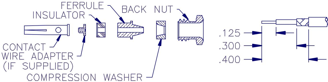
1. TRIM CABLE AS SHOWN. TIN END OF CENTER CONDUCTOR.
