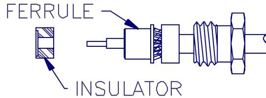
5. SLIDE FERRULE ONTO CABLE, OVER DIELECTRIC AND UNDER BRAID. PUSH INTO WASHER UNTIL IT STOPS. IF NECESSARY TRIM EXCESS BRAID FLUSH WITH SURFACE OF COMPRESSION WASHER AND FLANGE OF FERRULE.
