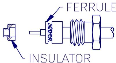
5. SLIDE FERRULE ONTO CABLE, OVER DIELECTRIC AND UNDER BRAID. PUSH INTO WASHER UNTIL IT STOPS. IF NECESSARY TRIM EXCESS BRAID FLUSH WITH SURFACE OF COMPRESSION WASHER AND FLANGE OF FERRULE.
