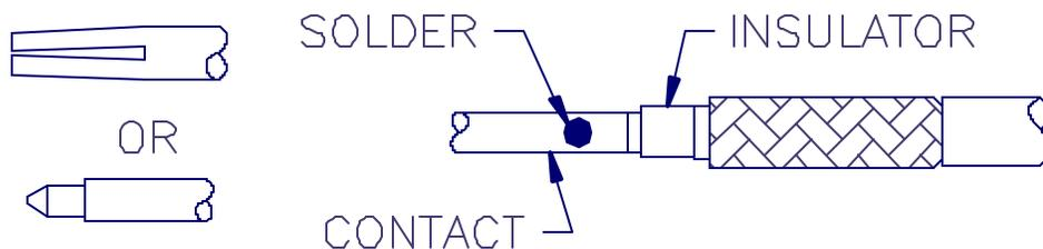
4. MOUNT INSULATOR AND SOLDER ON CONTACT.
