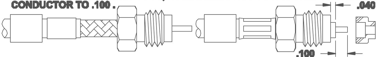
**3. SLIDE SHRINK SLEEVE FORWARD AND SHRINK IN PLACE AS SHOWN. INSERT INSULATOR OVER CENTER CONDUCTOR WITH STEPPED DOWN SECTION FACING OUT. SLIDE CONTACT OVER CENTER CONDUCTOR AND SOLDER IN PLACE. SCREW BODY ONTO CABLE ASSEMBLY. TORQUE TO 90-100 IN. OZ. (50 OHM).**
