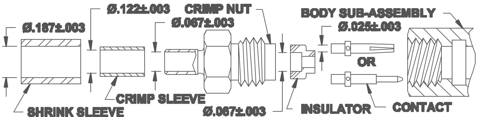
**1. SLIDE SHRINK SLEEVE AND CRIMP SLEEVE OVER CABLE. NOTE ALL DIMENSIONS ARE  $\pm .010$ . TRIM CABLE AS SHOWN. DO NOT NICK BRAID. TIN CENTER CONDUCTOR.**
