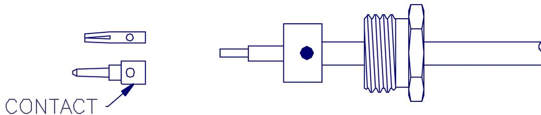
5. SOLDER CONTACT TO CENTER CONDUCTOR. CONTACT TO BE SEATED FLUSH AGAINST DIELECTRIC.
