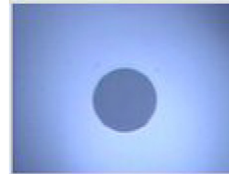
Connector end face after cleaning
