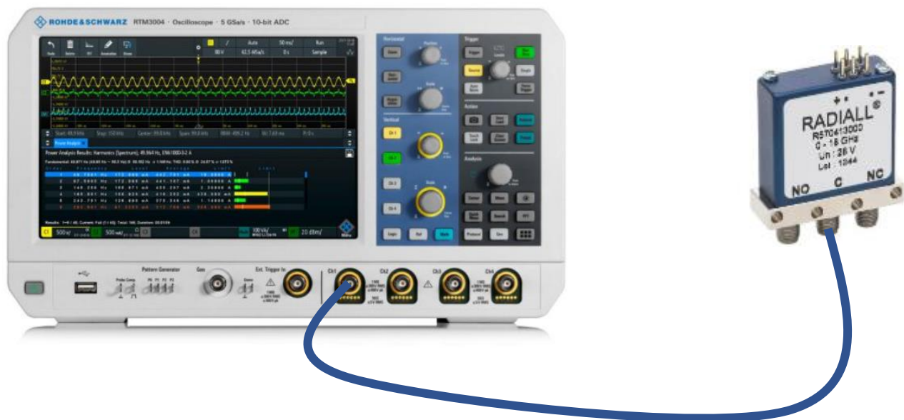
Figure 3: How to capture transients using high speed scope
