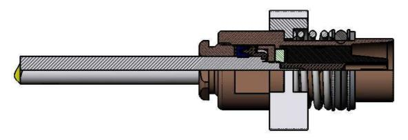
\*Picture above represents size 1 coaxial socket contact (620103) for display only.
