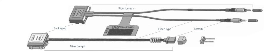
Module pigtail lengths are customizable from 10 to 50 cm with a typical tolerance of 15 mm. Tight tolerances are also available with a precision of 5 mm. Pigtails are strongly fixed to the module devices for high level of integration and robustness.
