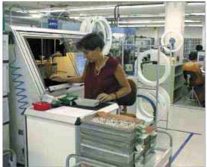
Connector manufacturing : press fit pins assembly line
