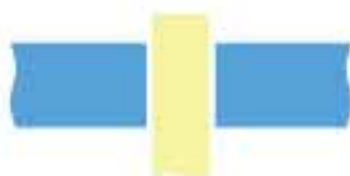
Dewetting case (wave soldering)
